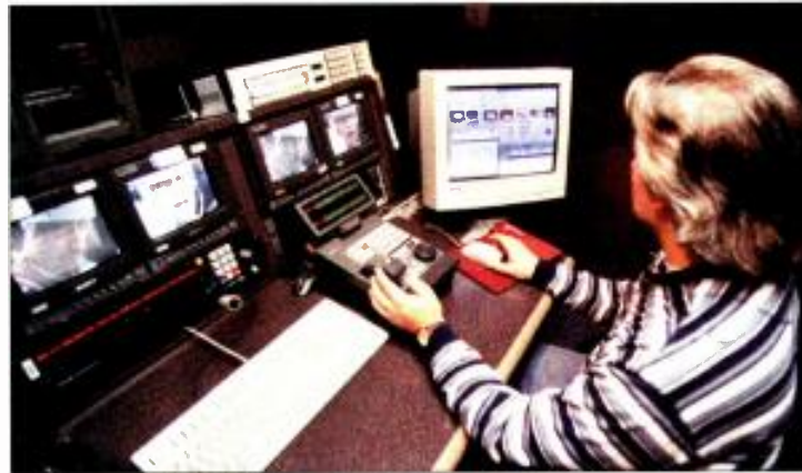
The Tektronix LVS live controller gives the Profile slo-mo capability. "It's really easy for our operators, who are used to slo-mo controllers for tape machines," says MSG's David Shaw.
